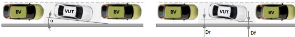
Fig. B.1 Schematic Diagram of Measurement of Deflection Angle (Left) and Distance from Curb (Right)
