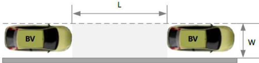
Fig. B.1 Schematic Diagram of Parallel Parking Space with Two Bordering Vehicles
