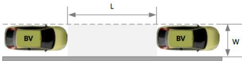
Fig. A.1 Schematic Diagram of Parallel Parking Space with Two Bordering Vehicles
